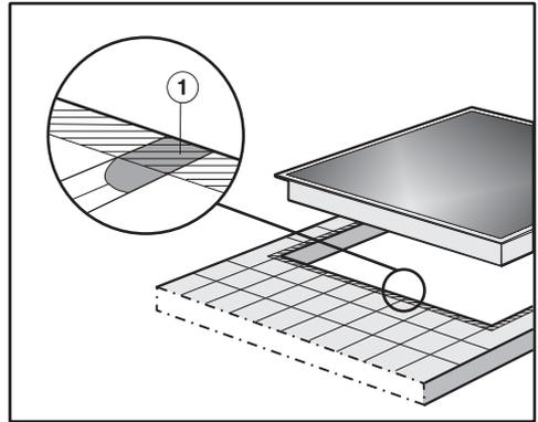
Grout lines ① and the hatched area underneath the cooktop frame must be smooth and even. If they are not, the cooktop will not sit flush with the worktop and the sealing strip underneath the cooktop will not provide a good seal between the cooktop and the worktop.
